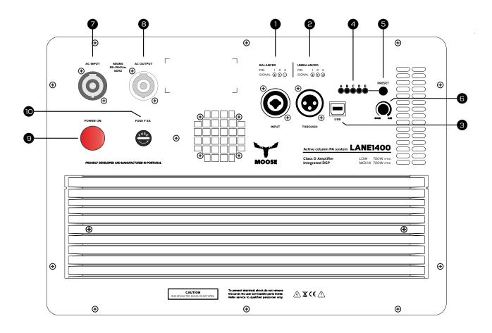
1. INPUT: Balanced signal input (Combi) for connection of an external audio source (e.g., mixer).
