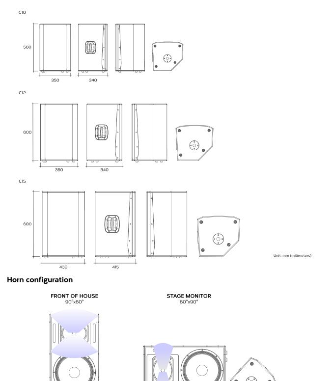
For Front of House configuration the narrow opening of the HF horn has to point downwards. For stage monitor configuration the HF horn has to be turned by 90 degrees, narrow opening pointing upwards. Remove the front grille and loosen the 4 screws of the HF horn. Turn the HF horn by 90 degrees and tighten the 4 screws. Then remount the front grille.
