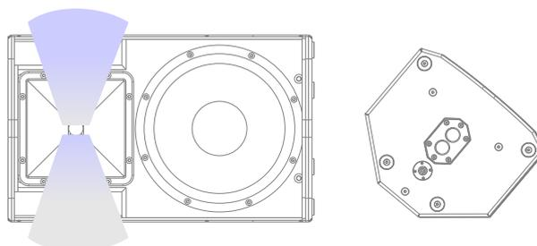
For Front of House configuration the narrow opening of the HF horn has to point downwards.
