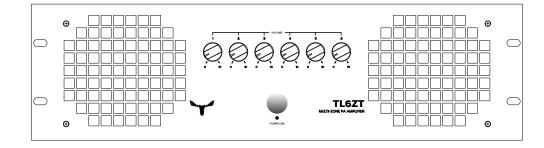
The TL6ZT is a Public address amplifier with 6 independent channels/inputs delivering each input 150W rms.
